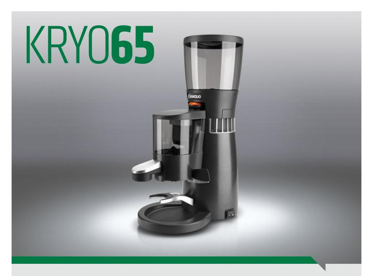
**KRY065** is fitted with 2.5 inch (64mm) diameter burrs, ensuring a production of 15-20 lb/h (7-9 kg/h). The dose can be regulated between 0.19 and 0.35 oz (5.5-10 g), with a coffee bean capacity of 2.9 lb (1.3 kg). It is available in an automatic (AT) or semiautomatic (ST) version.
